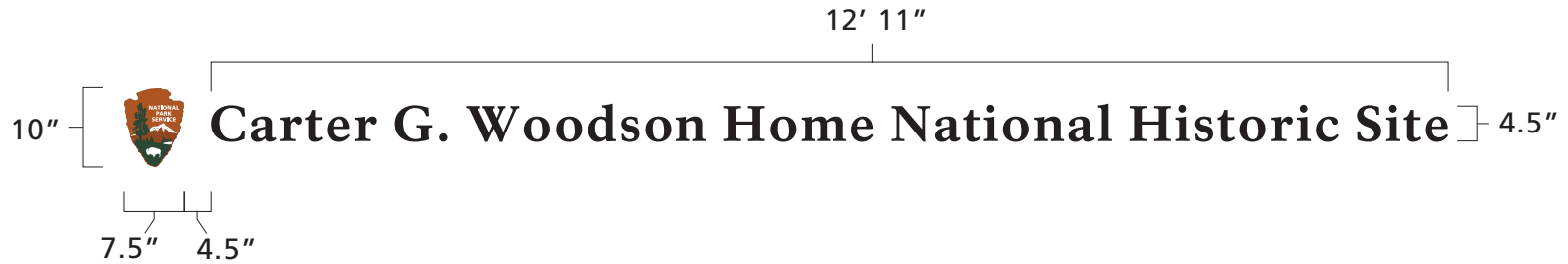
1.0 - Park Identity Sign - Painted Aluminum Arrowhead and Anodized Aluminum Pin Mount Lettering Scale: 1/2" = 1'-0"
